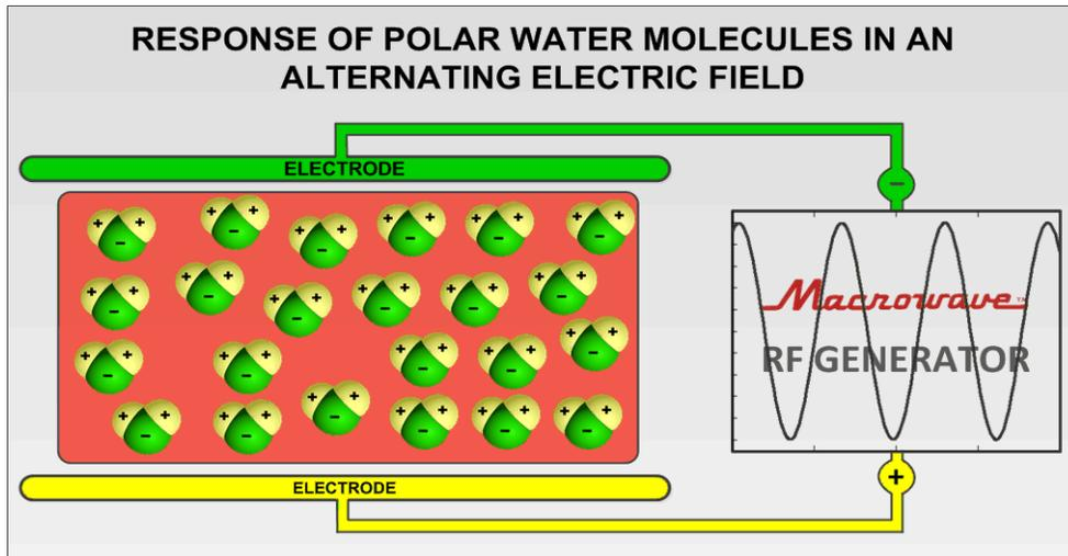
Macrowave™ systems operate within the approved 40.68 MHz radio frequency band width, which is an ISM (Industrial-Scientific-Medical) band width allowed for this type of equipment, as well as for medical devices commonly used for muscular diathermy. RF systems are appropriately shielded to meet with FCC regulations and the CE normative EN-55011. All units also comply with all OSHA regulations for safety.
