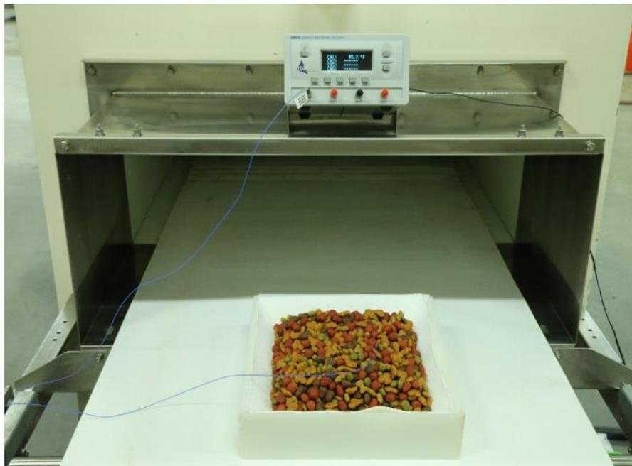
Successful functionality testing will show that the RF treatment process has had no discernable effect on any of the measured properties of the food item. At that time, moving into an inoculated challenge study is the next step in validating the process for that particular material.
